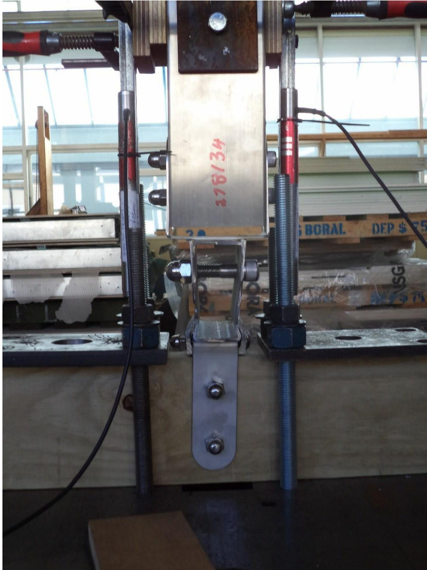
Photo 2. Specimen No. 278134 in test rig after failure had occurred.
